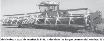
Moellenbeck says his swather is 14 ft. wider than the largest commercial swather. It's powered by a Caterpillar 3145 diesel and folds up for transport (below).
