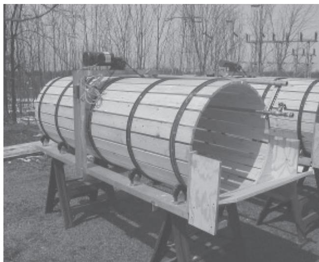
Rotating root washer is made from wood slats held together by steel bands, with gaps that allow water, soil and debris to run out.
