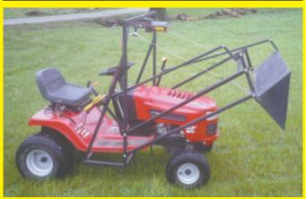
I've had a lot of response to your story on the high-lift mini loader I built for my garden tractor (Vol. 32, No. 3). The loader is operated by a 12-volt electric winch that hooks up directly to the tractor battery. A pair of levers or a 2-button control box are used to operate the lift and the power
