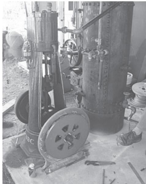
Normally, Dan Bartman uses the wind or the sun to charge up the batteries that let him live off the grid in Fort Collins, Colorado. But if he wants, he can burn wood to power a 1903 CB&H 6 hp steam engine that spins an alternator.
