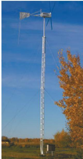
Alvin Troop put up this 5,500-watt wind turbine, called the Breezy 5.5, on a homemade 73-ft. tower.
