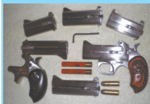
Interchangeable barrels allow this derringer-type handgun to shoot anything from a .410 shotgun shell to a full-size 45-caliber bullet.
