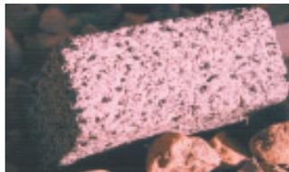
Bits of rubber from car tires, as seen on this block, boost concrete's insulation value and also deaden noise.
