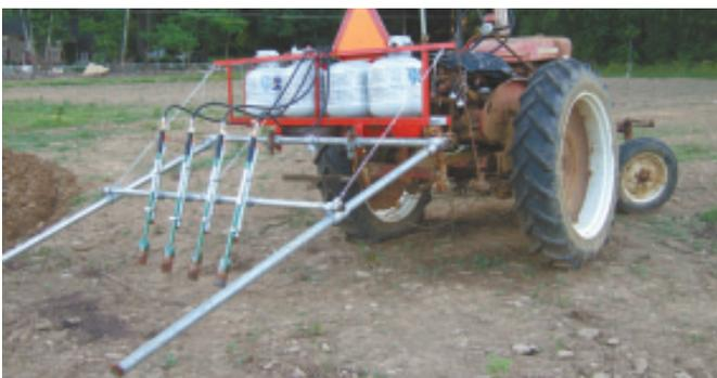
LP tanks are hooked up to four weed burners held about 8 in. off the ground.
