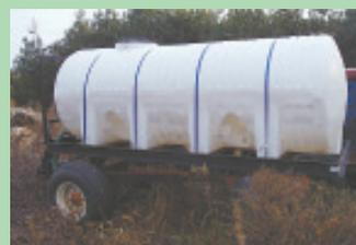
A 1,000-gal. tank on wheels has various sprinkler head options.
