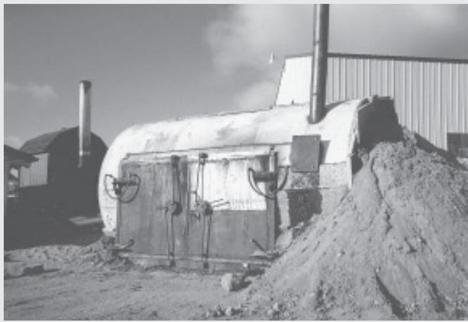
Louie Shively used a 10,000-gal. fuel tank to build this giant outdoor wood stove. Back side of stove is banked with dirt for insulation.
