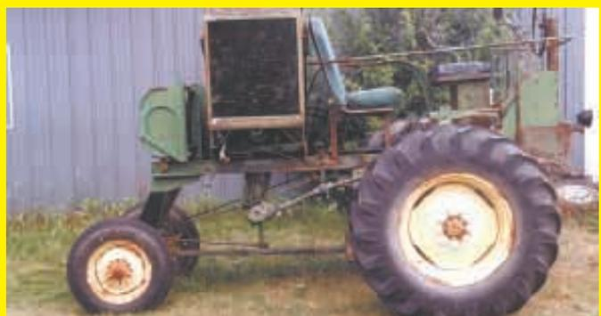
I needed an extra tractor to pull wagons to the field. I didn't want to spend the money for another tractor so I made my own by cutting down a 1953 model 55 Deere combine. I shortened the frame 4 ft. and used angle iron to reinforce the frame. It still uses the original belt drive to the transmission. I added a school bus
