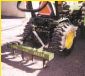
Here's a photo of a 4-shank ripper that I made for my Deere 4110 compact yard tractor. I bought a used 4-ft. box blade and cut off the box blade part, leaving a framework on which I mounted the four ripper teeth. Works great for ripping up any large garden area. I spent less than
