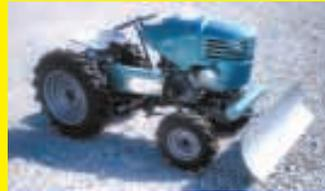
This photo shows a Speedex model 17 garden tractor equipped with a front-mounted snow blade, which I recently restored. I installed a new 10 hp electric start motor and added new tires and paint. The tractor has a 2-speed transmission, with one forward gear and one reverse. The engine slides forward to tighten the belt, and is pulled back to put on the brakes by using a foot pedal.
