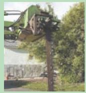
Trimmer can be pivoted to a vertical position to cut the sides of hedges.
