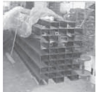
Compartments each measure 5 by 7 in. and are set up in a "checkerboard" pattern, to reduce the amount of tubing needed.
