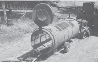
Maurice Leighton modified a commercial "Billy Goat" vacuum by replacing the bag with a higher-capacity drum collector. He pulls it behind his riding mower.
