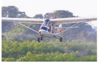
QuickSilver's ultralight crop sprayer has a matching controlled droplet spray system.
