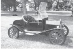
Half-scale Model T car is powered by a Honda 5 hp gas engine. "Our grandkids have lots of fun with us driving this car," says Dale Lemmerman. "Top speed is about 15 to 20 mph."
