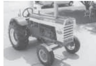
The tractor is complete with a set of half size gauges that Scott bought at Wal-Mart, and the muffler was purchased from a farm supply store. Apilastic bowl was used to make the air cleaner.
