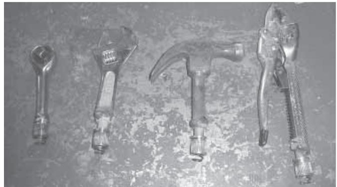
To use shop tools with his prosthetic arm, Matt Biel cut the handles off the tools and then welded a bolt onto each one. Then he threaded special adapters onto the bolts.
