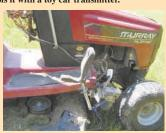
He installed a reversible 12-volt motor to control the steering wheel through a pulley and belt system (left). Another motor controls forward and reverse on the transm
