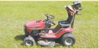
Jones mounted a video camera on his riding mower. Video is transmitted back to the TV in his house with a router device normally used for networking computers together.
