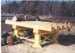
Table is designed so two operators at the same time. one at each end of table, without having to bend over. The operator cuts through log at every space between the timbers.
