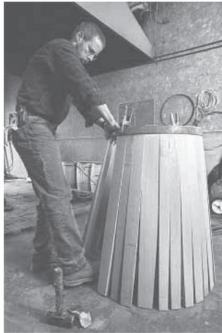
Barrels are made with lengths of tapered stave wood, bent and held together with steel hoops.
