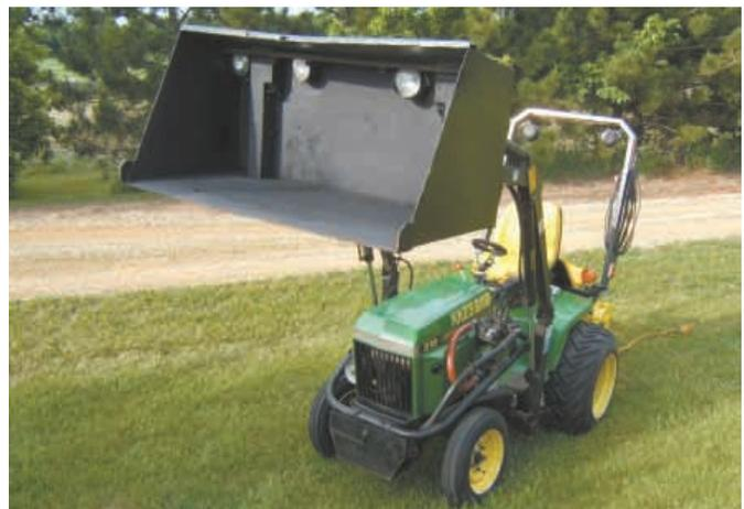
Deere 318 garden tractor is fitted with a Johnson Workhorse loader and an extra large, 1,000-lb. capacity bucket for snow and dirt. Note headlights at upper part of bucket.
