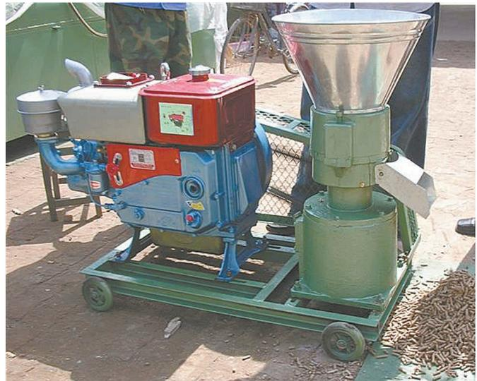
Pellet Pro pelletizer mills range in output from 65 lbs. an hour to a turnkey, 2-ton per hour system with dryer/cooler and bagger.
