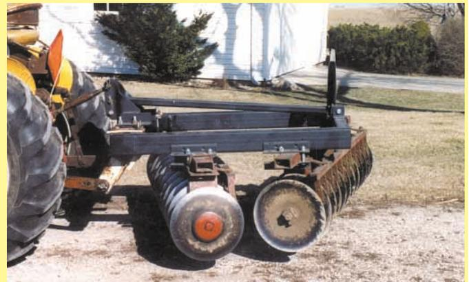
Ben Hach built this 3-pt. mounted, 7-ft. offset disk from an old tandem disk.
