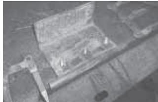
**Homemade jig allows cutting and welding the broken guards together.**
