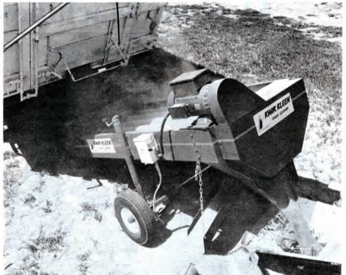
The cleaner is made up of five 6-in. dia. perforated screen cylinders, each 6 ft. long and placed side by side.
