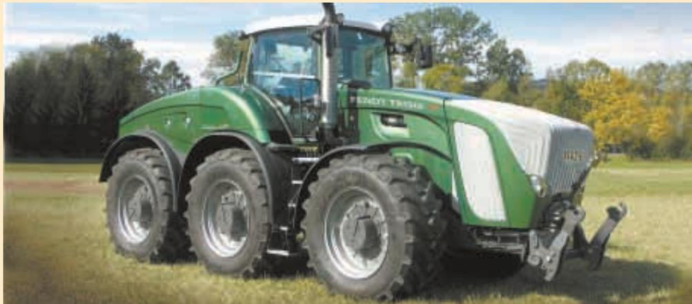
Prototype 6-wheel, triple axle AGCO tractor features a 540 hp engine, yet it's only 9 ft. wide.
