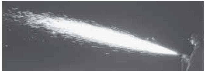
What looks like a flame is actually a steel alloy melted with a 14,000-volt-amp power source and then sprayed using almost 5 cu. ft. of air per second.
