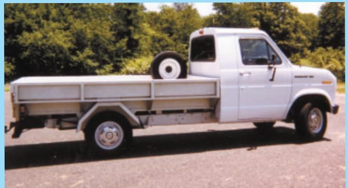
A heavy-duty pickup with a 10 1/2-ft. long bed. That’s what Bruce Mossbrucker got when he converted a 1985 Ford E-350 1-ton van. The extra long cargo box has a multi-level bed.
