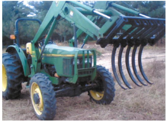
Tree “fork” was made by mounting five old chisel plow tines on a rectangular metal frame, which quick-taches to the loader on Ezra’s Deere MFWD tractor.
