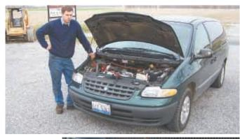
Mark Steiner pulled the gas engine out of his Plymouth car and dropped in a 2.2-liter Isuzu diesel. He had to cut the frame rails to make the engine
