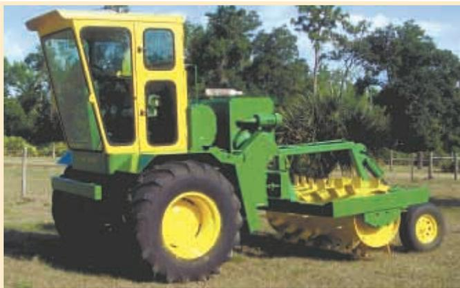
Farrell Johnson built this self-propelled machine to take on compacted soils.
