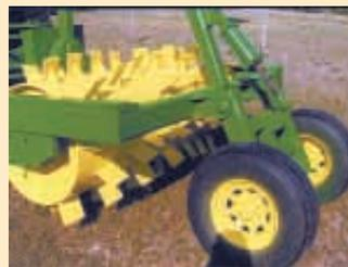
Filled with water, the 30-in. dia. drum is heavy enough to penetrate and open heavily compacted ground.
