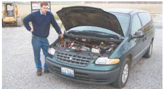
Mark Steiner pulled the gas engine out of his 1997 Plymouth car and dropped in a 2.2-liter Isuzu diesel. He had to cut the frame rails to make the engine fit.
