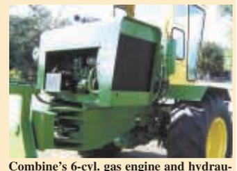
Combine's 6-cyl. gas engine and hydraulic pump mount behind the cab to provide down pressure on the aeration drum.
