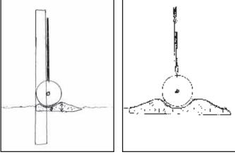
Wheel at bottom of gate rides up over concrete hump and settles into a "cup" against a backstop (left). The same idea can be used on gates that open both ways (right).
