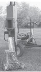
Fence post pounder is fitted with a homebuilt splitting axe attachment.
