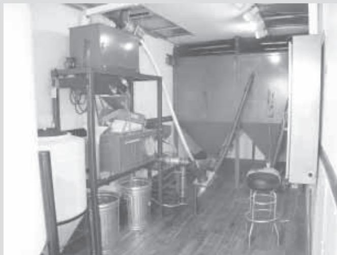
**Unit can produce 80 gal. of canola oil every 24 hours and extrudes the leftover canola meal into pellets, which can be fed to cattle or used in a pellet stove.**
