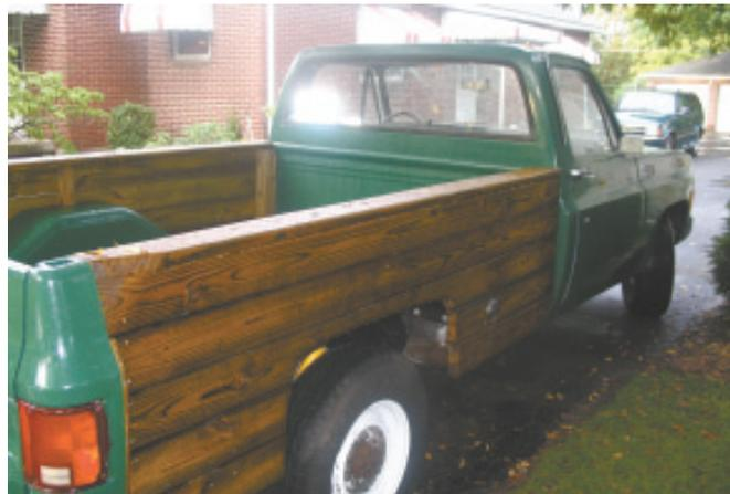
**After he couldn't find replacement side panels, Wolters built his own wooden sides for the bed on his Chevrolet 3/4-ton pickup, using pressure treated 2 by 6 pine boards.**
