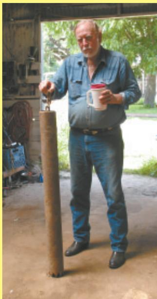
**Home-built well cleaner has teeth at the bottom that stir up sediment so it can be pulled out.**
