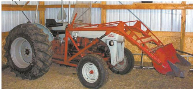
To keep the original tires on his Ford 8N from sinking in wet ground, Leon Lease fitted it with 16.9 by 26-in. combine wheels.
