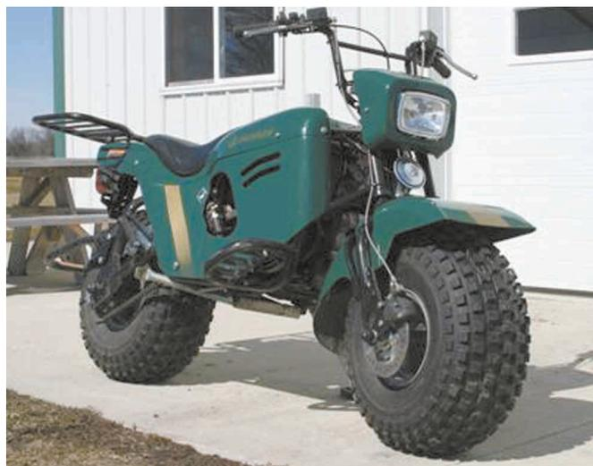
According to the company, the Ecorider's 11-in. wide tires cause less damage to the ground than a person on foot so you can drive over wet ground with minimal damage.
