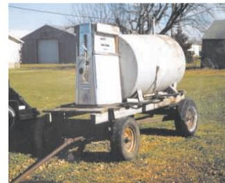
To collect used oil from others, Lou Holland mounted a 500-gal. tank on a 4-wheel cart along with an older-style gas station pump.
