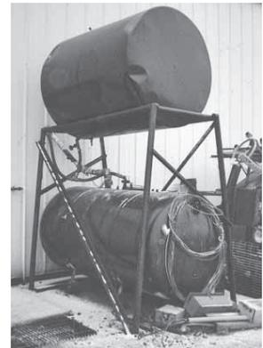
**When the storage drum inside is full, oil is pumped to a pair of 300-gal. storage tanks outside the shop.**
