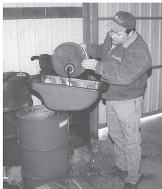
**Connecting an old tractor oil pan to a barrel makes it easy to dump used oil, says Mike Miller.**
