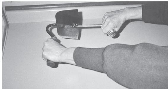
Two-handed edger uses garden hoe blade to cut.
