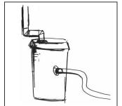
Spencer used thermostat housing to fasten a hose to the garbage can.
