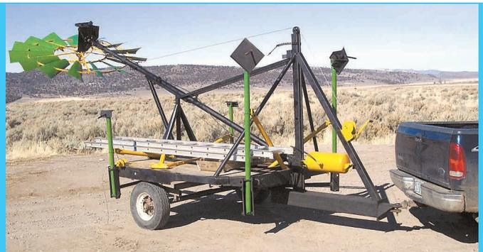
Jack Vernon's portable pneumatic windmill folds down for transport on a 2-wheeled trailer, allowing him to transport the windmill at highway speeds between remote pastures.
