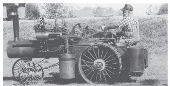
It took Arnold Green three years to finish this half-size working model of a 20 hp Advance Rumely steam engine. It has one speed forward and one speed reverse.
