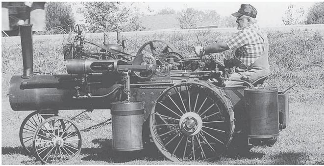
It took Arnold Green three years to finish this half-size working model of a 20 hp Advance Rumely steam engine. It has one speed forward and one speed reverse.
