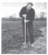
"Bait stick" tube has a spring-loaded base. It meters out bait as base is pushed against a hole.
