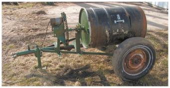
Holst's 55-gal. composter rides on the running gear from an old cattle loading chute. An old silo distributor turns both the shaft and drum for mixing.
