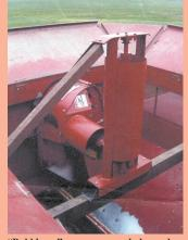
"Bubble up" auger was made by replacing the original cross fill auger with an auger that just goes to the center of bin. There, it fastens to a right angle gearbox which then drives another auger that goes straight up.
