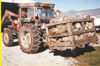
hydraulic cylinder in place of the top link on my tractor's 3-pt. hitch. I built a mounting bracket for the cylinder and use a lever to extend or retract it. The stabilizer chains have to be kept tight to prevent side sway. (Perry Hathaway, 4238 W 625 South, Claypool, Ind. 46510 ph 574 491-3448)
