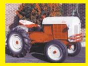
I built a 1/2 scale Ford 8N. I got the hood, grill, and fenders from Don Knasel who makes a mini Ford kit (www.awesomehenry.com). I built the little tractor from a Cub Cadet, adding a Ford 8N seat and a cutdown dash. It has a 16 hp engine. It took about 2 months off and on to build it. (Stanley R. Wolf, 714 Black Horse Tavern Rd., Gettysburg, Penn. 17325 ph 717 334-2444)
