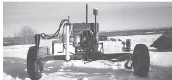
Two-in-one machine has a wood splitter on one side and a welder on the other.
