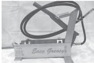
Grease gun holder lets you pump the grease gun with one hand or foot.
