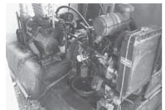
Air power unit consists of a 40 hp diesel engine that belt-drives a line shaft, which in turn drives an air compressor, a hydraulic pump, and a blower that takes sawdust away from Weaver's saws.
