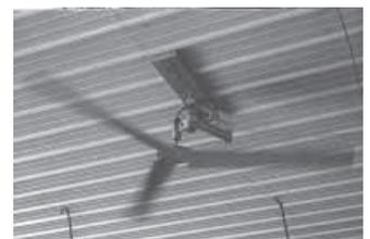
Weaver uses air to power a large ceiling fan in his shop. Compressed air is directed through a line mounted at ceiling level to an air motor above the fan.
