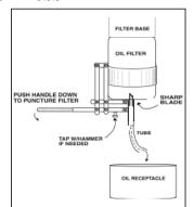
Tool slips over bottom of filter and pokes a hole in it to drain away the oil inside. If spear won't penetrate filter, you can use a hammer to tap on metal knob next to spear.
