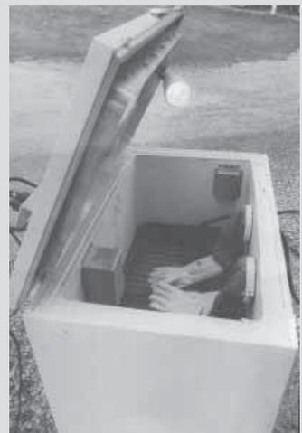
Leather welding gloves, sewed to pant legs, extend inside freezer.
