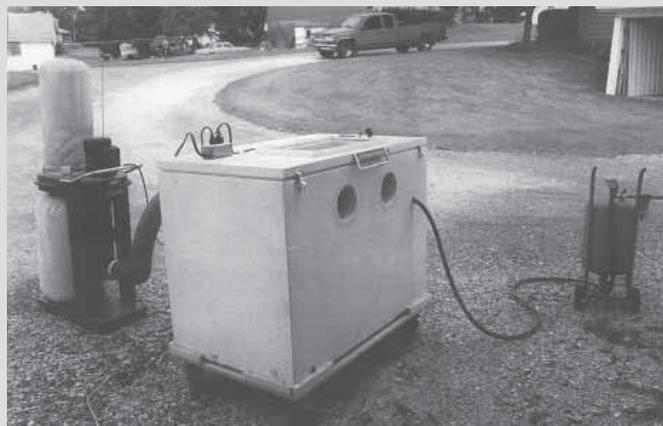
Casey Grant came up with the idea of using a deep freezer as the cabinet for his sandblaster. Blaster at right hooks to air compressor.
