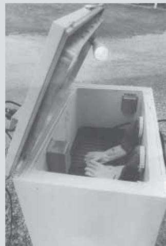
Leather welding gloves, sewed to pant legs, extend inside freezer.
