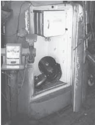
**Rex Gogerty, Hubbard, Iowa:** "An unused old refrigerator provides dust-proof, moisture-proof storage for planter units, monitors, etc. I installed a latch on the door
