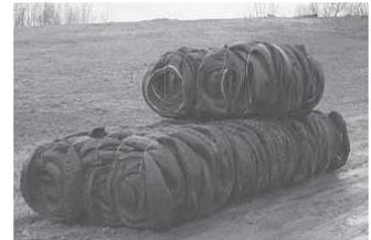
Tire bales provide great insulation, can act as load-bearing walls, and are virtually indestructible. They can be easily stacked and require no stabilizing structure around them.
