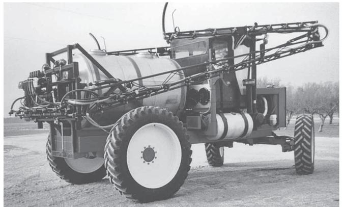
Koehler's sprayer is equipped with a 1,200-gal. stainless steel tank off a John Blue sprayer, as well as an 80-ft. hydraulic-fold boom equipped with nozzles on 20-in. spacings. He paid \$12,000 for the combine at an implement dealer.
