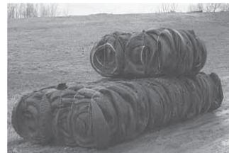
Tire bales provide great insulation, can act as load-bearing walls, and are virtually indestructible. They can be easily stacked and require no stabilizing structure around them.
