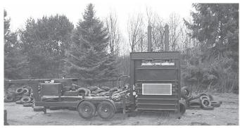
Tire baler packs 100 car tires into a brick 30 by 50 by 60 in. that weighs about a ton. Five 9-gauge galvanized or stainless steel baling wires hold each tire brick together.
