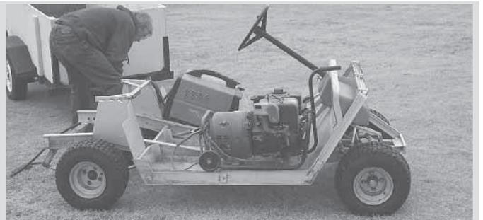
Burns mounted a generator, hydraulic power pack, and a welder on an old golf cart.
