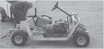
Burns mounted a generator, hydraulic power pack, and a welder on an old golf cart.
