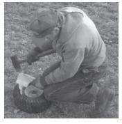
Paul made the bead breaker out of an old car wheel rim and scrap metal. "Just one strike of the sledge hammer and the bead is released," says Paul.
