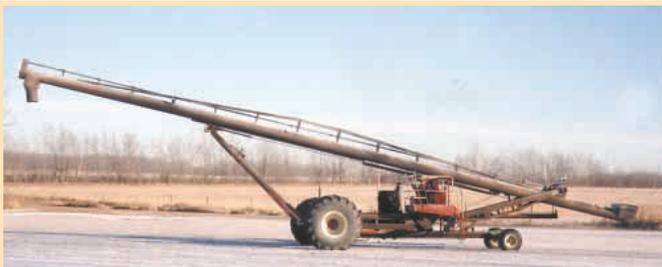
Beamish spent about 500 hrs. building this 13-in. dia. auger that's 60 ft. long and has a capacity of about 9,300 bu. per hour. It's mechanically driven by a 6-cyl. 251 Chrysler industrial engine through a gearbox from an 8650 White pull-type combine.
