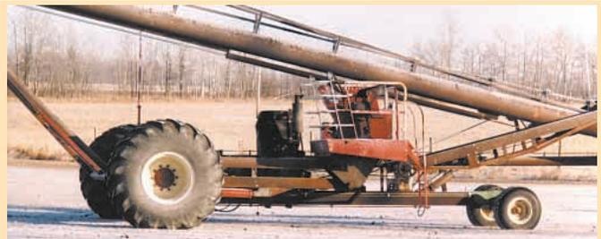
From the platform, Beamish can maneuver the rig and control auger height.
