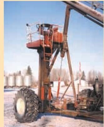
"The whole reason for the moveable platform was to make it easier for positioning the auger at the top of the bins," Beamish says. "The platform raises up 12 ft. and moves forward about 8 ft."
