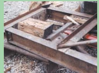
A 4 by 24-in. hydraulic cylinder pushes against a 30-in. wide steel wedge that does the splitting.
